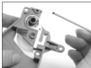
Each remanufacturing cycle, remove conductive grease from the metal contact in the gear housing end plate. Apply a small amount of conductive cartridge lubricant (Item Code: CON-CLUBE) to the contact.
