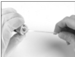
Clean toner, grease and debris from the contact prongs on the mag roller sleeve. Use a cotton swab dampened with isopropyl alcohol.
